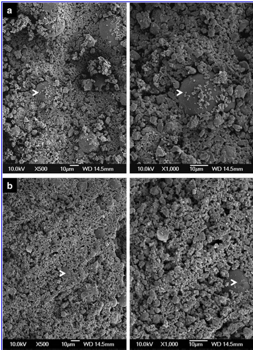
**FIG. 3.** Scanning electron micrographs. **(a)** CPC containing PLGA microsphere at 500 $\times$  and 1000 $\times$  magnification; **(b)** CPC containing PLGA microspheres and DCA at 500 $\times$  and 1000 $\times$  magnification. Arrows indicate PLGA microspheres.
