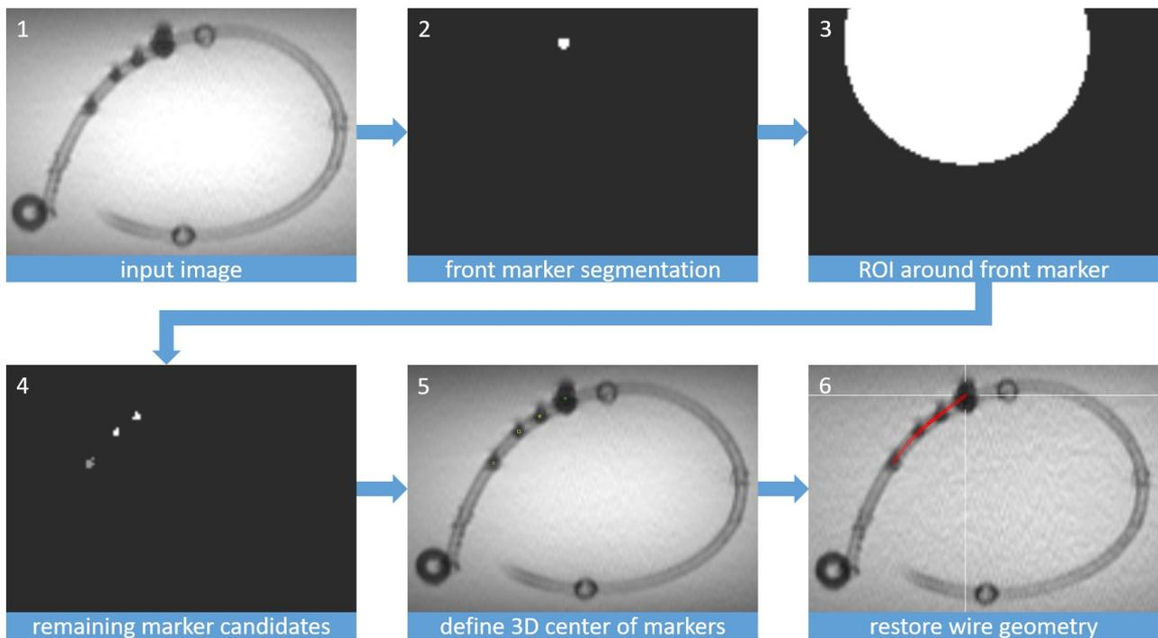
Figure 2: Overview of the wire reconstruction: (1) input image, (2) front marker segmentation, (3) limit search radius for subsequent algorithms, (4) segmentation of remaining markers, (5) define centers of gravity and (6) find best approximation.
